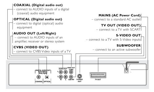
Caution: Do not touch the inner pins of the jacks on the rear panel. Electrostatic discharge may cause permanent damage to the unit.
